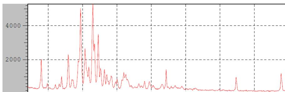
**Figure No 7: X-ray diffraction of pure Ezetimibe**
