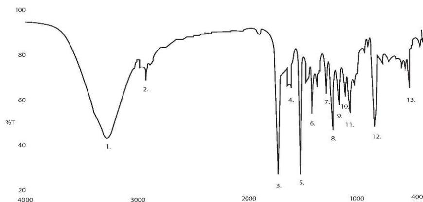
**Figure No 6: IR spectra of LS formulation-F4**
