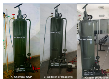
Figure 3: Plant in use: A-Prototype plant; B-Chemicals being fed : C-O2 being produced
