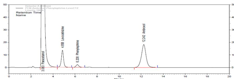
Fig. 5: Chromatogram of blank and Standard for specificity
